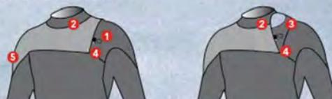
1. ZIPLESS ENTRY SYSTEM: Water tight seal with ease of entry and exit.
